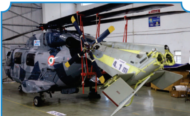
The Demonstration of the tail boom folding operation was carried out on November 7, 2020 on ALH Mk-III DWDM prototype helicopter.
